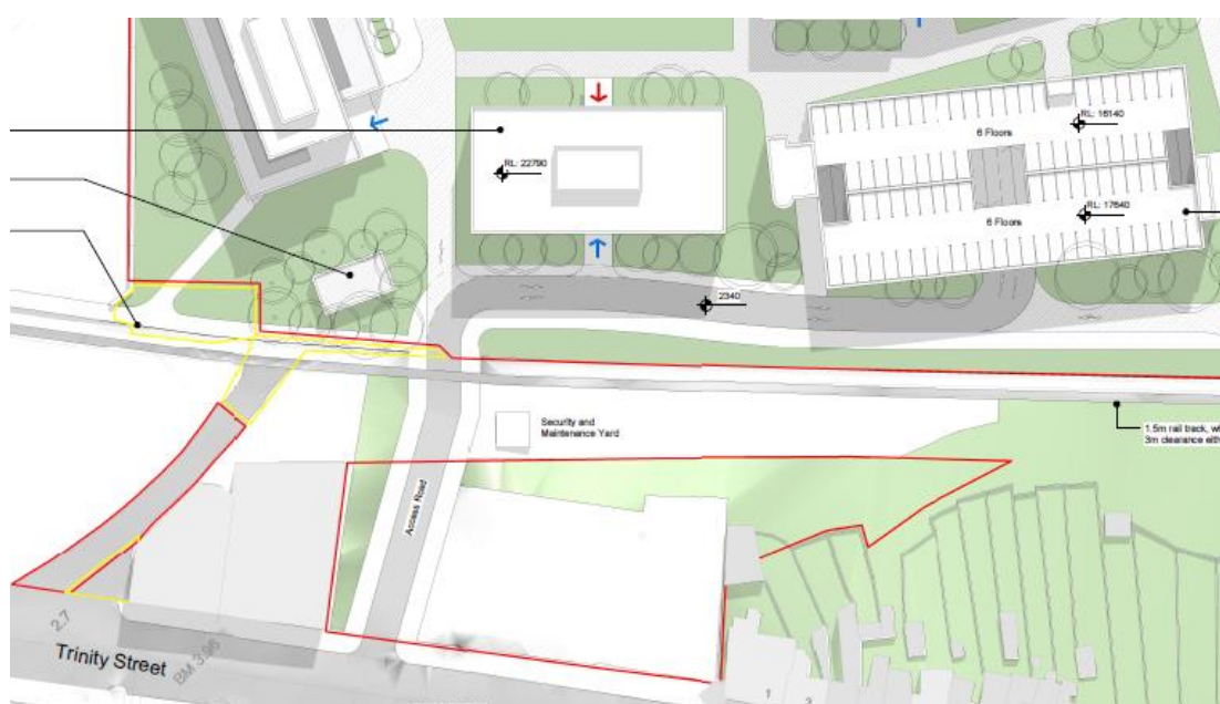
Plate 3.8 Straight access road alignment (Note: the site layout in this plate is taken from the conceptual design stage and contains elements including the site boundaries, have been updated as part of the final design)
